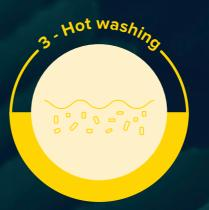
An upgrade from standard cold washing, flakes are hot washed to remove organics, adhesives, inks, and other contaminants.
